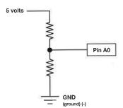
A voltage divider consists of two resistors. The "top" resistor is the sensor you'll be using. The "bottom" one is a normal, fixed resistor. When you connect the top resistor to 5 volts, and the bottom resistor to ground. The voltage at the middle will be proportional to the bottom resistor relative to the total resistance (top resistor + bottom resistor). When one of the resistors changes (as it will when your sensor senses things), the output voltage will change as well!
